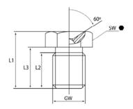
SW = Wrench Size L1 = Total Length L2 = Thread length L3 = Shank Length GW = Thread All measures in mm
