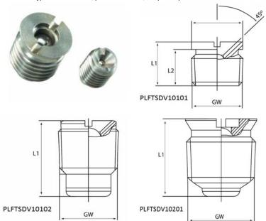
L1 = Total Length L2 = Thread length GW = Thread All measures in mm
